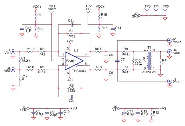
**Note:** Devices designated with an \* are not installed on the EVM. The user must supply these components.
